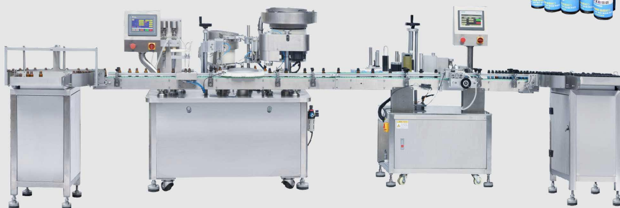
理瓶转盘 Bottle arranging turntable
