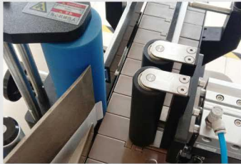
气缸夹瓶定位机构 Cylinder clamp bottle positioning mechanism
