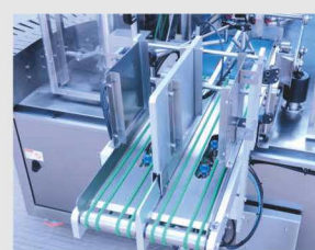
双袋仓 (一次供两袋) Double bag bin (for two bags at a time)
