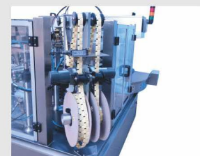
双袋干燥剂投包 Double bags of desiccant package
