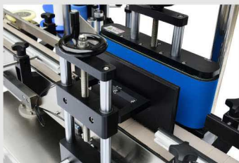
搓滚式覆标机构 Rolling type label covering mechanism
