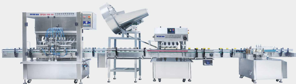
八头气动直线自动活塞式广口瓶灌装/上盖/旋盖/浆糊贴标生产线 Eight-head pneumatic linear automatic piston filling wide mouth bottle filling/capping/capping/paste labeling production line
