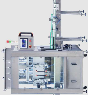
双头活塞式跟随灌装机 Double-head piston type follow filling machine
