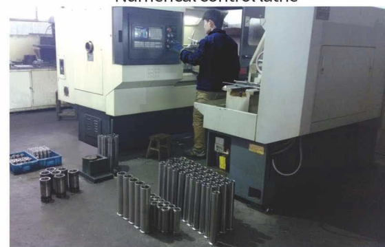
活塞缸精密加工 Precision processing of piston cylinder
